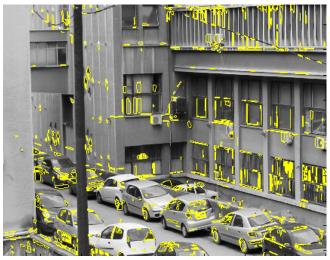
Fig. 9. Detected MSER features in example image
